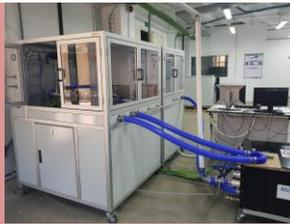
ENSAYOS PILA DE HIDROGENO 100 KW
